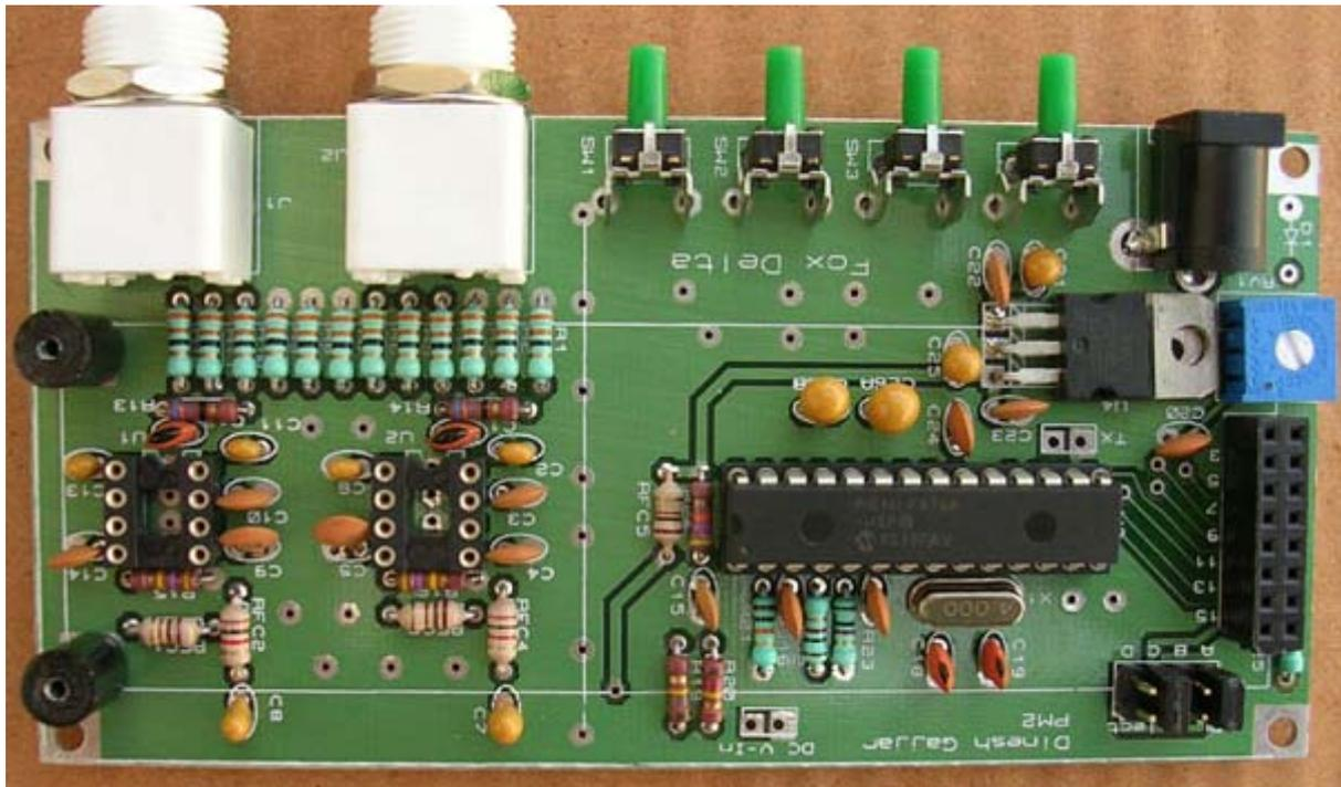
I do not supply AD8307 with this kit for simple reasons. First, they are bit expensive and second, not everybody may require two channels for RF measurement. Moreover, most hams may register with [Analog Devices](#) & obtain AD8307 as Samples.
