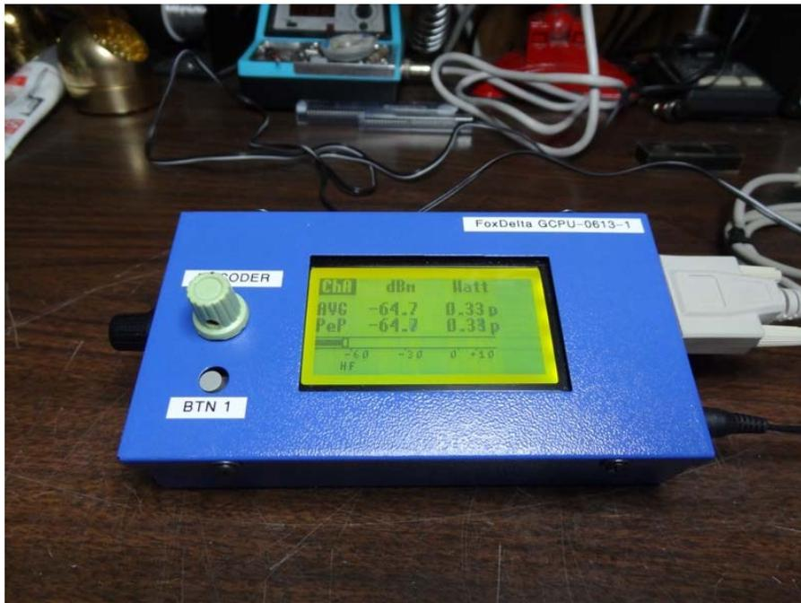
3. Press “BTN 1” once to switch the unit into the HF-VHF-Custom (CST) Frequency Range.
