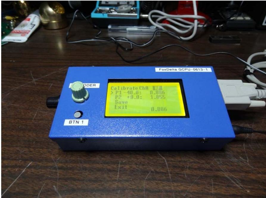
10. Press “BTN 1” and Cursor on LCD Display should move next to “P2” 0.0 dBm Calibration point. Adjust your Calibrated Signal Source to 0.0 dBm, but do not change frequency. See FIGURE 6
