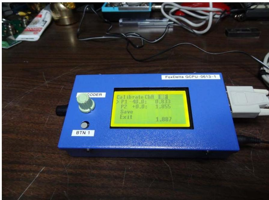
9. Press (Push) the ENCODER Knob, and you will see the numerical value at the bottom of the LCD display has been inserted into the “P1” -40 dBm calibration point. See FIGURE 5.
