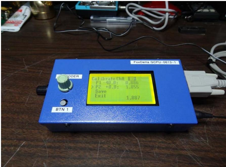
11. Note numerical value representing 0.0 dBm displayed at the bottom of the LCD display. Press (Push) the Encoder Knob and this value will be transferred into the “P2” 0.0 dBm Calibration point. See FIGURE 7.
