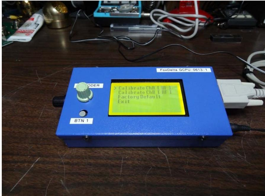
8. Press (Push) ENCODER Knob and you should see the Calibration A HF Screen shown in Figure 4.
