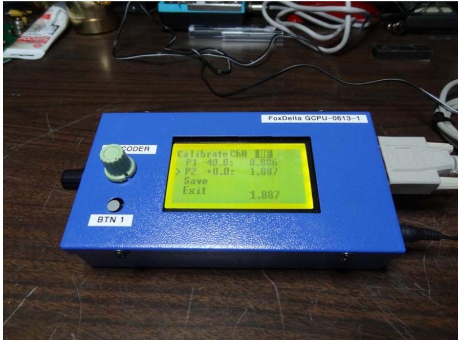
12. Press “BTN 1” and the Cursor should move next to “SAVE”. Press (Push) the ENCODER Knob and the “SAVE” line will blink “SAVE CALIB” several times as the Data is saved in the HF measurement mode.
