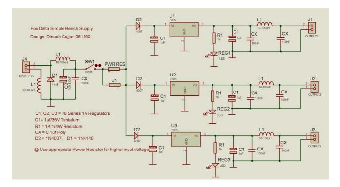
J4 is the input connector where we will apply any available voltages from 5V to 24V (or beyond). J1 is a jumper or a fusible low ohmic resistor.
